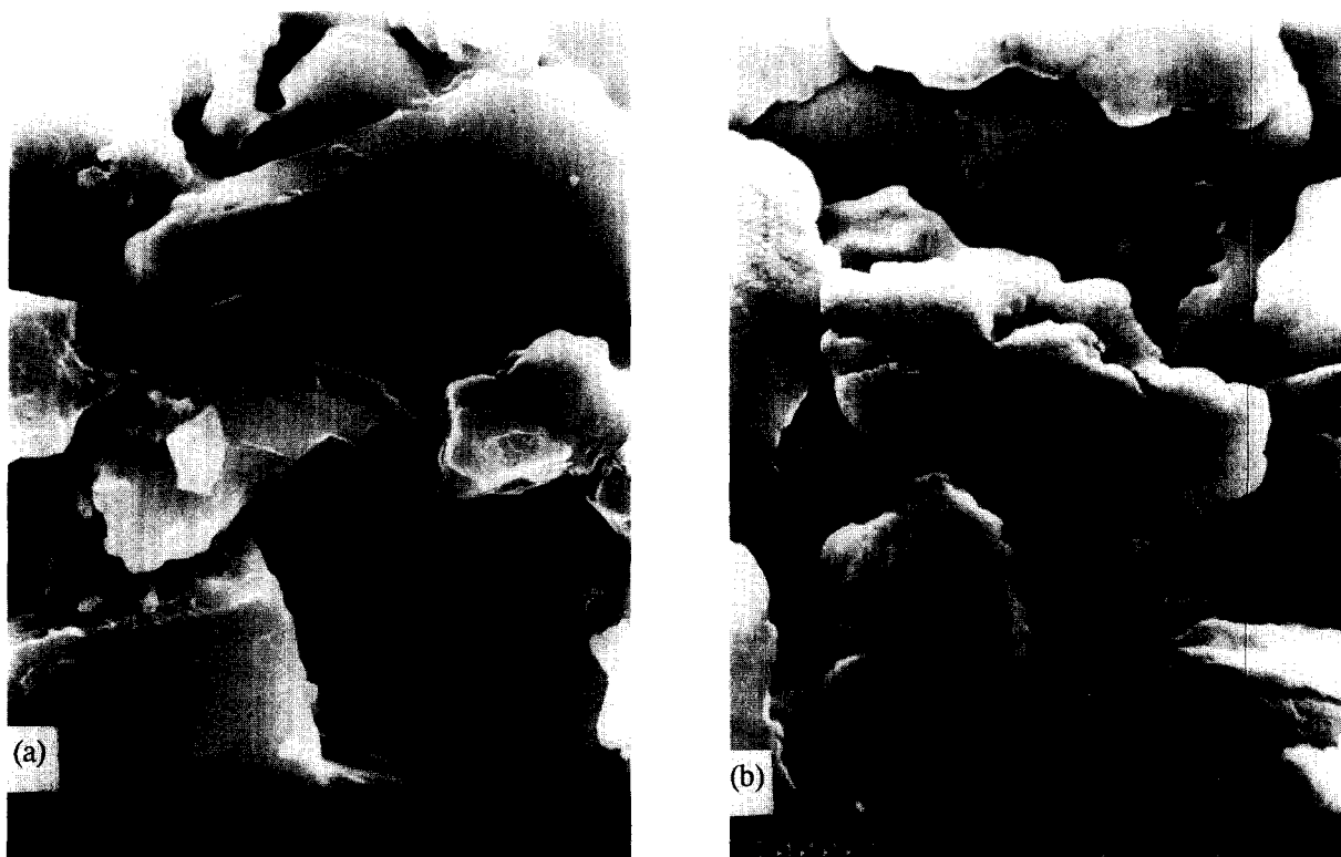
Fig. 1. SEM photographs of the \alpha - \text{Al}_2\text{O}_3 support tube ( \times 10\text{ K} ): (a) outer surface; (b) inner surface.
